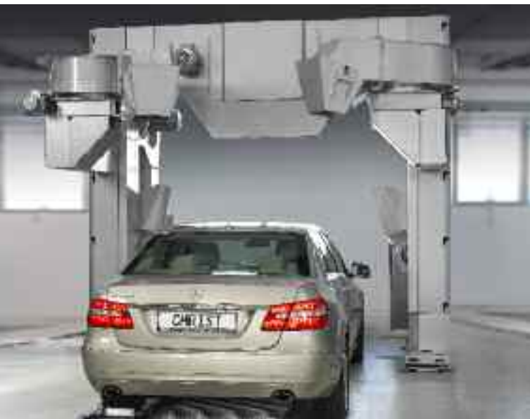
Start setting: Air stream directed against vehicle's front
