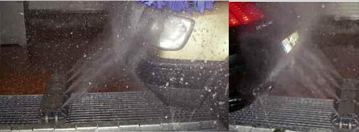
Medium-pressure spray device for front, under-body and rear, floor installation above-ground
