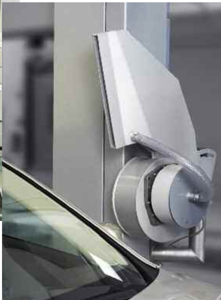
VAN Dryer For drying optimization on the upper side areas of higher vehicles (can be switched on according to the height of the vehicle). The VAN Dryer is mounted on the basic frame of the drying blower AEROFLEX between the roof blower and the side blower. It consists of two blowing devices, each with a blowing motor and can be manually set in height, inclination and angle.
